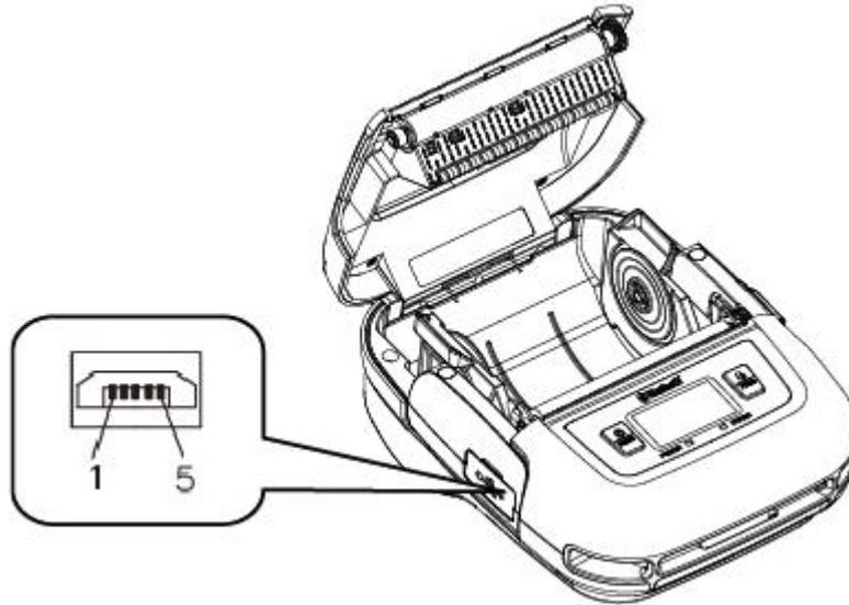
iMOVE T3Pro printer has a USB interface for Battery charging and is connected by means of 5pin micro USB socket. In the following table, the signals present on the micro USB socket are listed.
