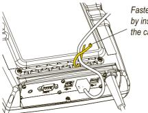
Fasten cables to the 8515 by inserting cable ties through the cable management bar.
