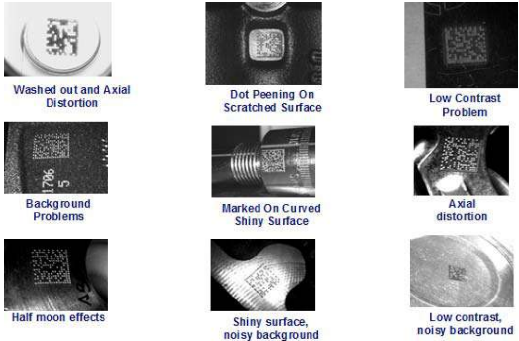
Figure 85 - Problematic Direct Part Marking Examples
