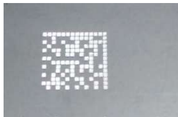
Figure 26 – Dot Peening Marking on Metal Surface with Multi-dot per Code Element
