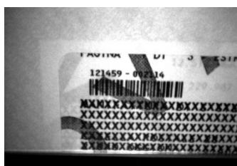
Figure 23 - Overprinted Barcode Readable by Matrix 410N also Through the Envelope Window Film
