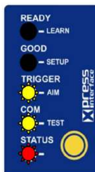
Figure 9 - X-PRESS Interface: Aim Function
