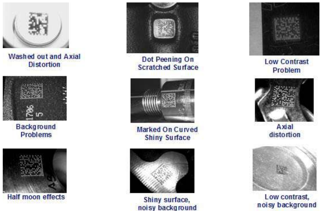
Figure 84 - Problematic Direct Part Marking Examples
