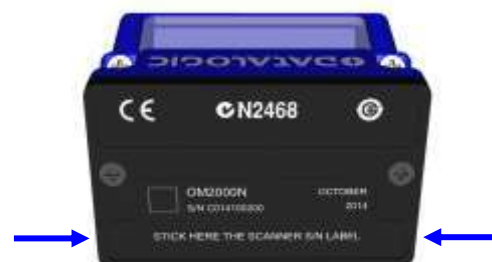
Figure 35 – Apply Replicate Scanner SN Label
