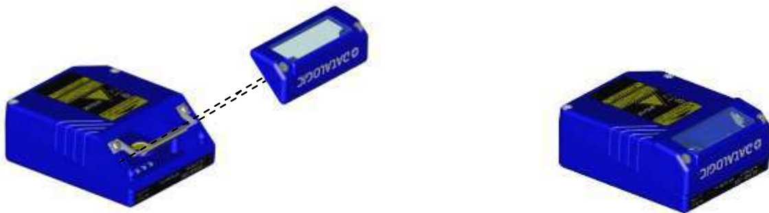
Figure 19 - Mounting a GFC-2020 Deflection Mirror
