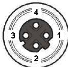
Figure 93 - M12 D-Coded Female Ethernet Network Connector
