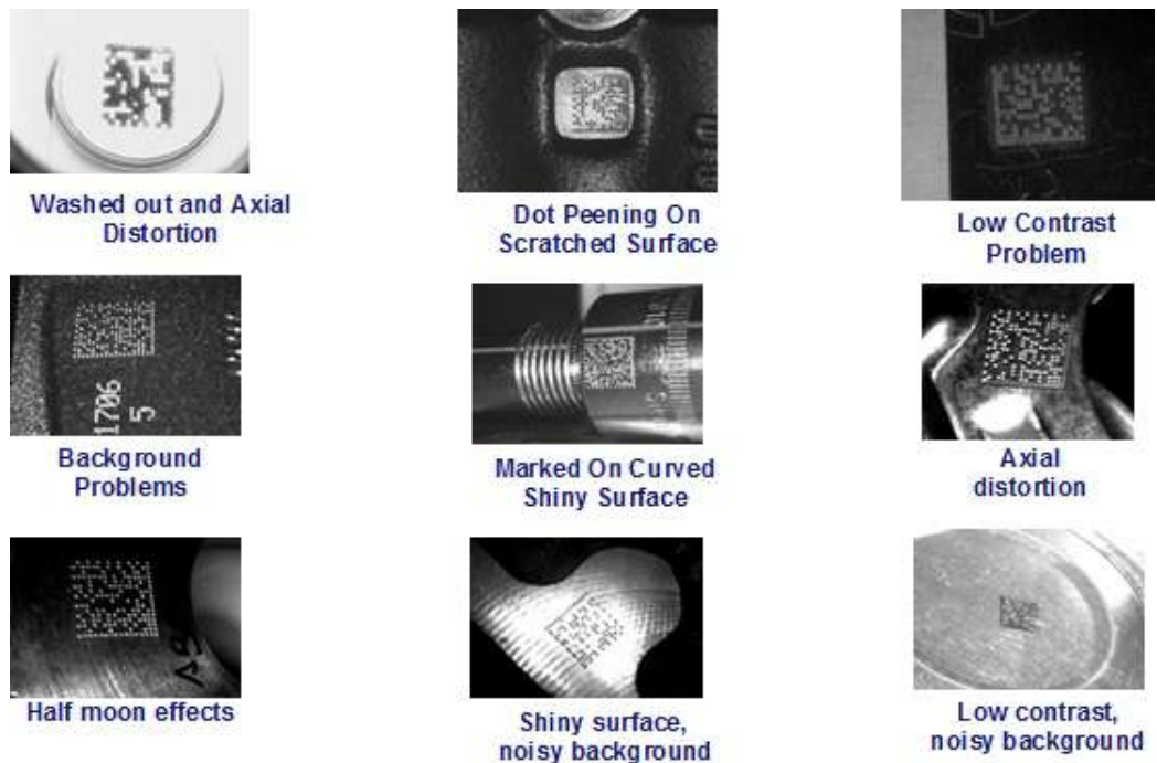
Figure 93 - Problematic Direct Part Marking Examples
