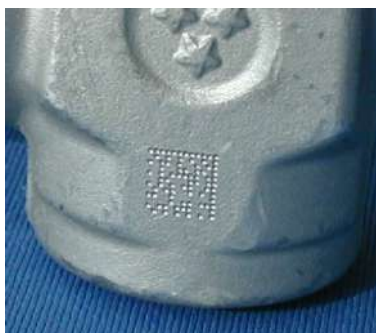
Figure 23 – Dot Matrix Code Directly Marked on Metal Surface by Using Dot Peening Technology
