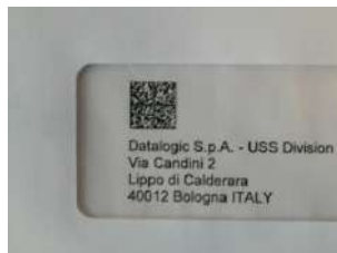
Figure 18 - Address Coded in Data Matrix Symbology for Automated Mail Processing
