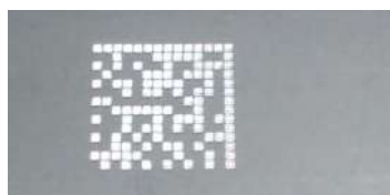
Figure 24 – Dot Peening Marking on Metal Surface with Multi-dot per Code Element
