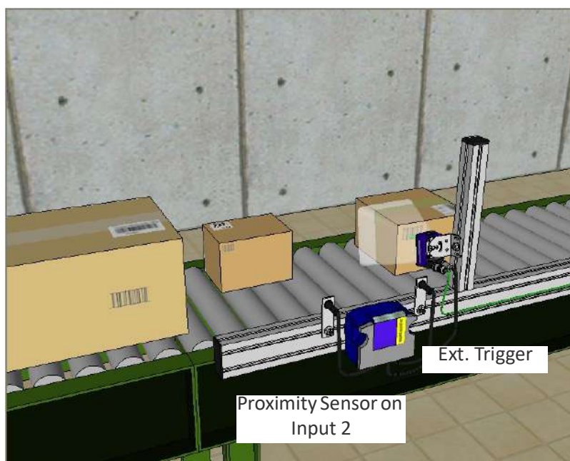
Figure 92 - Example Extending DOF Using External Image Settings Selection
