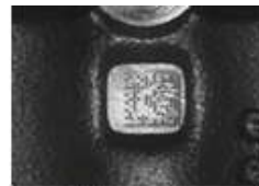
Dot Peening On Scratched Surface
