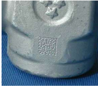
Figure 20 - Dot Matrix Code Directly Marked on Metal Surface by Using Dot Peening Technology
