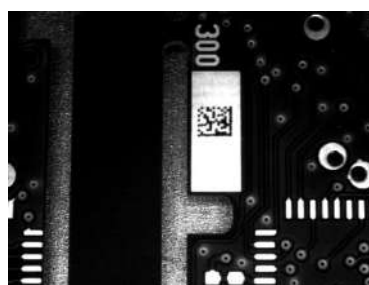
Figure 24 - Dot Matrix Code Directly Marked on PCB Copper Pad by Using Ink-Jet Technology
