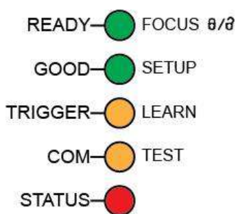
Figure 9 – X-PRESS Interface: Focus Lock/Unlock Function
